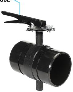
Model B8200 Buttlerfly Valves are available in sizes 2 through 8 inch diameters. Precision machined grooves in the valve body provide easy alignment of the valve and compatible PVC couplings, allowing for the insertion of the spline to connect the Model B8200 Valve to the PVC piping system. Flow may enter the valve from either direction and valve can be orientated in any direction.
